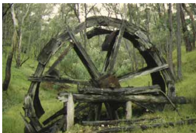
Figure 6.29: Water wheel, a key structure used to power huge stamping-battery machines, part of the heritage-listed Weone gold mine, Victoria
