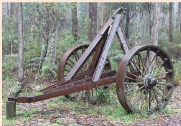
Figure 6.31: Bobtail used for pulling logs out of the forest, Lowden Forest Park, New South Wales
