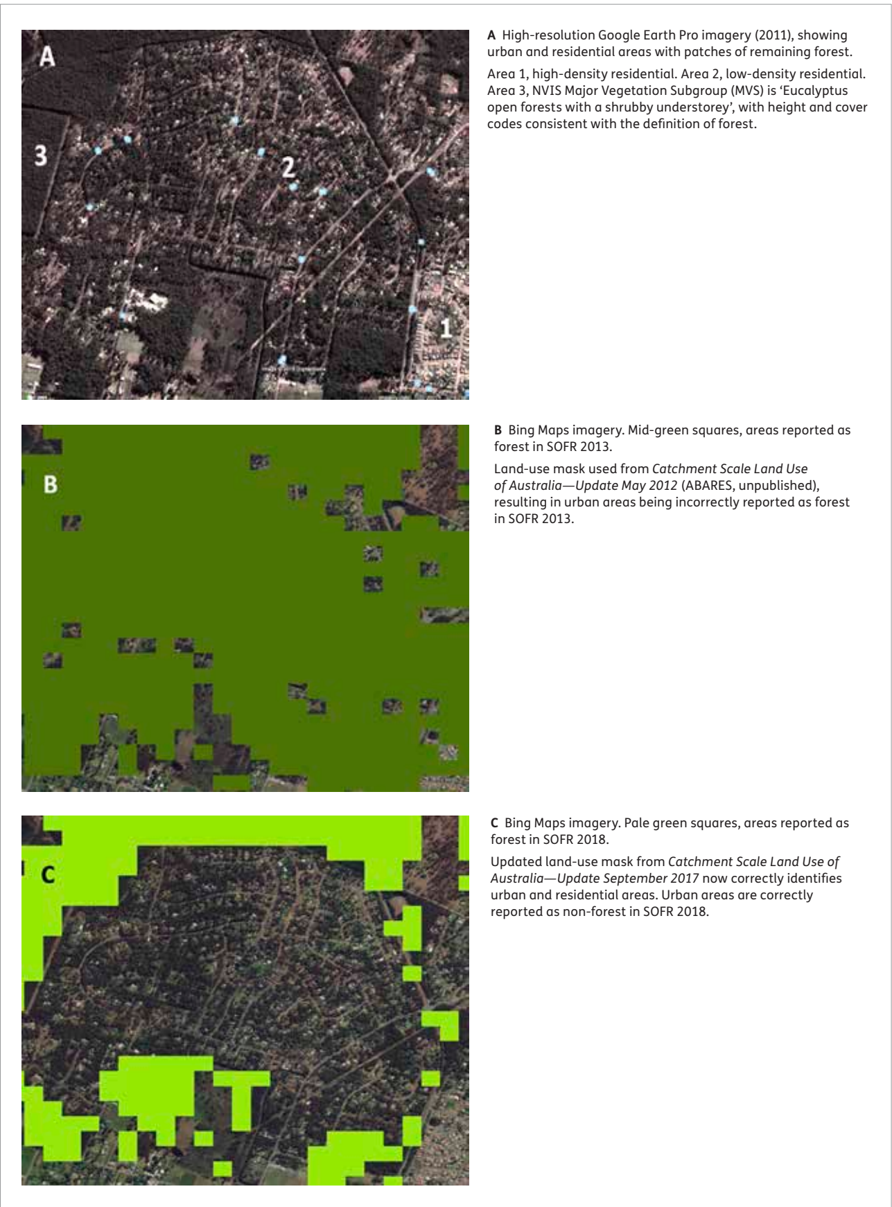
Figure 1.10: Example of an area reported as forest in SOFR 2013 but as non-forest in SOFR 2018 due to application of an updated land-use mask. Medowie, north coast New South Wales. Individual mid-green and pale green squares on images B and C have an area of 1 hectare (100 m x 100 m).
