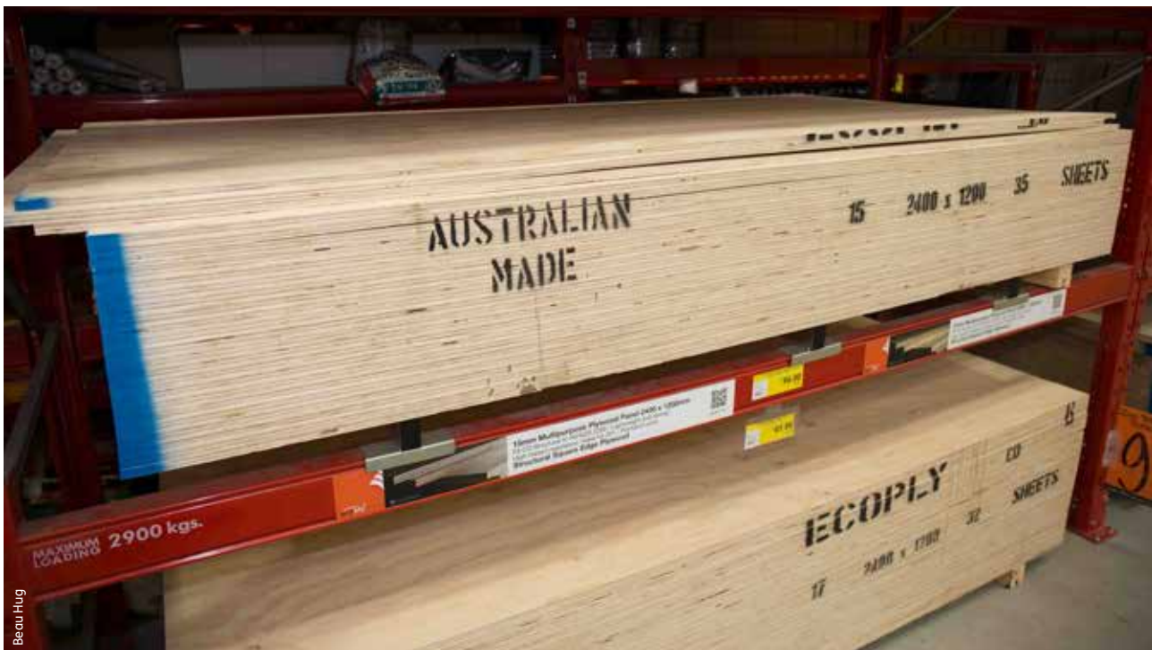
Structural-grade plywood made in Australia from plantation pine.
